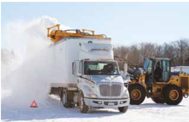
It takes less than a minute to clear snow from a tractor-trailer or bus with TrucBrush.
